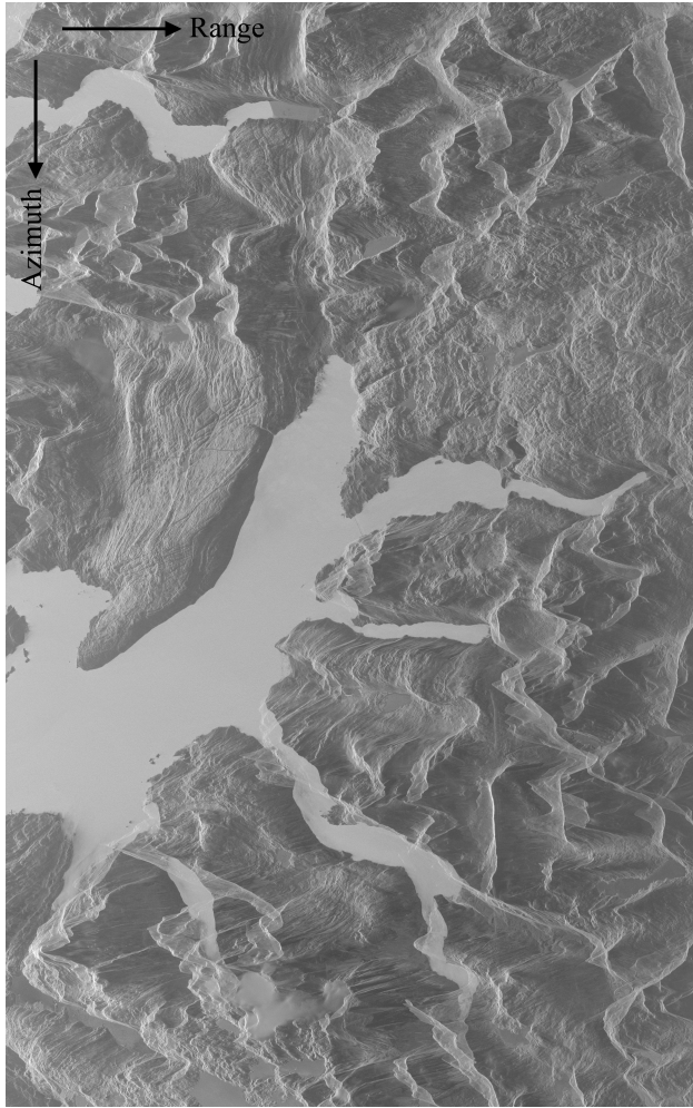
Fig. 1. An image acquired in Stripmap mode from ICEYE SAR satellite constellation over the Ofotfjord in Norway on February 24th, 2020 (size approximately 40 km x 70 km)
