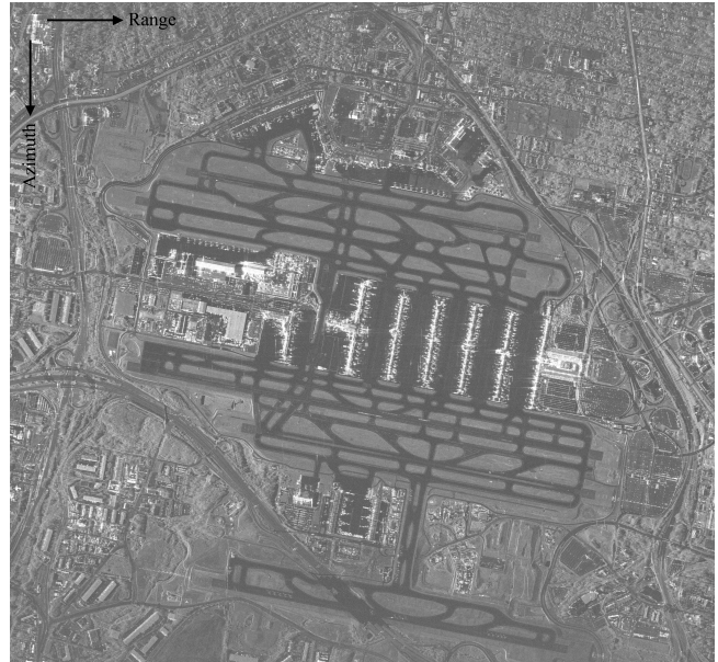
Fig. 2. A Spotlight image with 25 cm of resolution from ICEYE SAR satellite constellation over the airport of Atlanta in USA on March 24th, 2020 (size approximately 5 km x 5 km)
